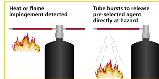
We have various sizes of tubing that ranges from very slim and flexible enough to coil around electrical panels to heavier tubes connected to pipework, structured around larger more industrial equipment, all designed to detect and suppress at the very source of the fire.
